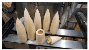
Joe Garofalo - Hand-threaded nose cone rocket box. Threading demonstration was on AAW. Super glue in threads, let it dry, then again, then paraffin.
