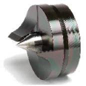
"Spur drives" suitable for such use in a four jaw scroll chuck are available from Craft Supply or Oneway Manufacturing among others. Craft Supply calls them "Quick Change Drive Centers" like p/n 361-0102 (see left). It is recommended to use the two spur drive, vs. the four, for driving bark or irregular bowl blank surfaces as these dig deep into the grain when lined up in the same direction.
