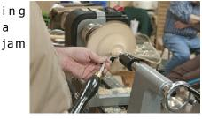
chuck, he proceeded to remove the While removing the tenon, tenon. he slightly undercut the foot area.
