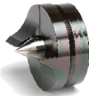
"Spur drives" suitable for such use in a four jaw scroll chuck are available from Craft Supply or Oneway Manufacturing among others. Craft Supply calls them "[Quick Change Drive Centers](#)" like [p/n 361-0102](#) (see left). It is recommended to use the two spur drive, vs. the four, for driving bark or irregular bowl blank surfaces as these dig deep into the grain when lined up in the same direction.
