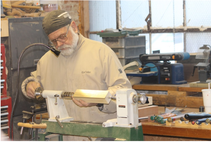
Jim centering the wood on the lathe
