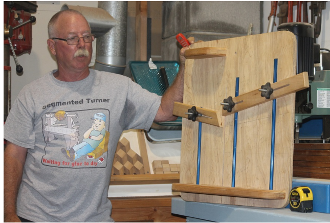
Butch with a jig he made and uses for cutting segmented pieces
